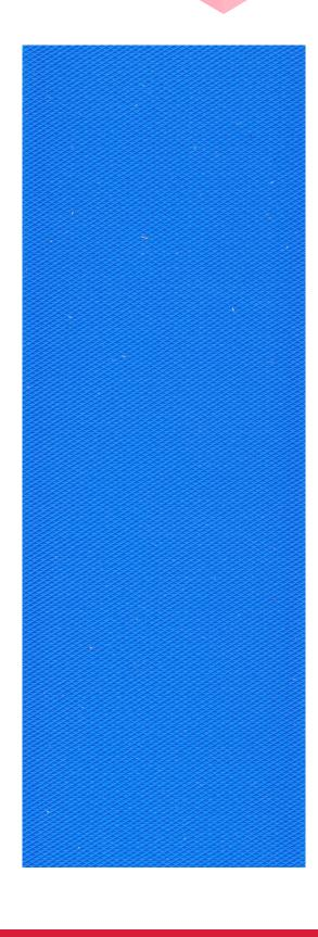
Special coated wrap knitted fabric, flexible in cross direction and stiff lengthwise, thin with high tenacity.
